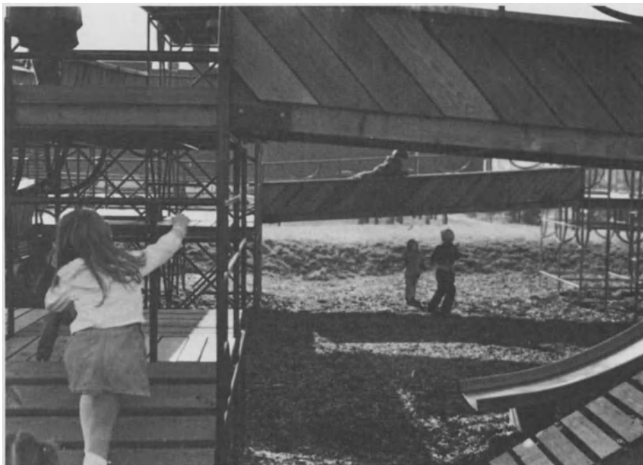
The Heights Playstructure. The continuous ramp spirals up 11 feet, forming a hollow "hill," limiting falls to short distances on the outside, and creating a "meeting place" on the inside.
