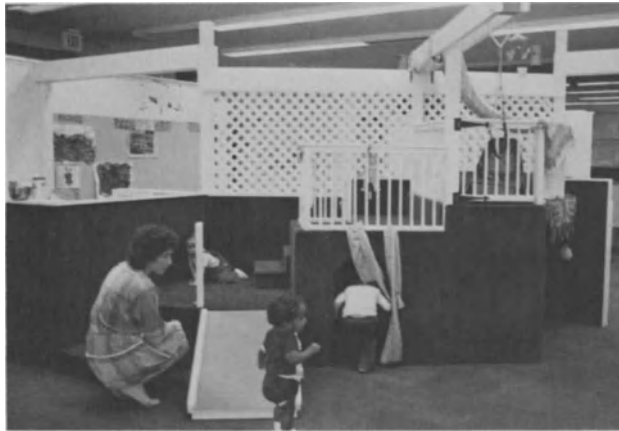
FIGURE 2. The infant group side of a dividing wall which incorporates a slide, stairs to climb, semienclosed and fully enclosed upper levels, an underneath crawl space, a beam from which to suspend gross motor apparatus, a diaper-changing area, and lattice work permitting visibility to the toddler side.
